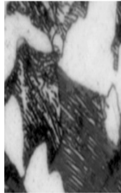
Ferrite and more blackish Pearlite grains at 0.4% C
