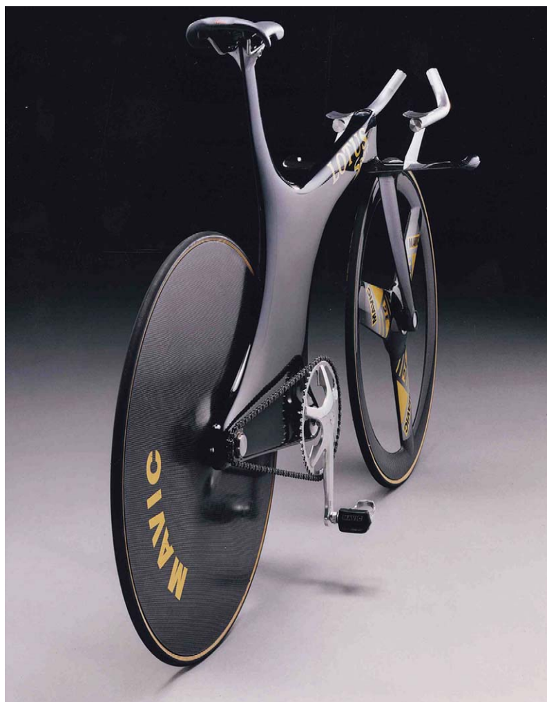
Carbon fiber-reinforced plastics were at the heart of this bike built by Lotus Engineering for the 1992 Barcelona Olympics. It helped Chris Boardman win gold. (Courtesy of Lotus.)
