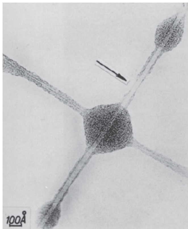
Viewgraph showing a single- or double-walled CNT published in 1976. (Reprinted with permission from Oberlin, A., et al. , J. Cryst. Growth (1976) 32 , 335. © 1976 Elsevier.)
